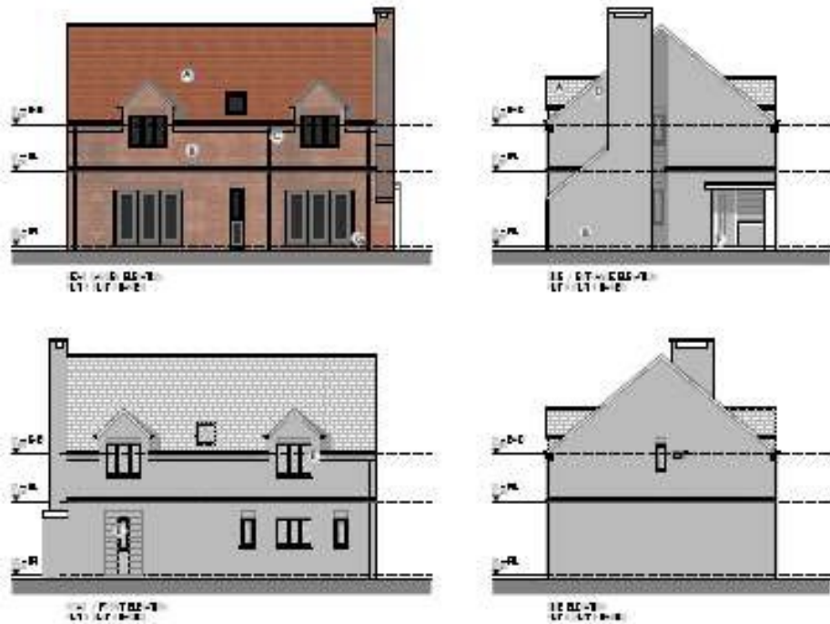
Figure 9: Cottage form: Low eaves (and ridge) with through-eaves windows; brick with brick detailing and clay plain tiles to roof. Powder coated composite aluminium / timber windows.
