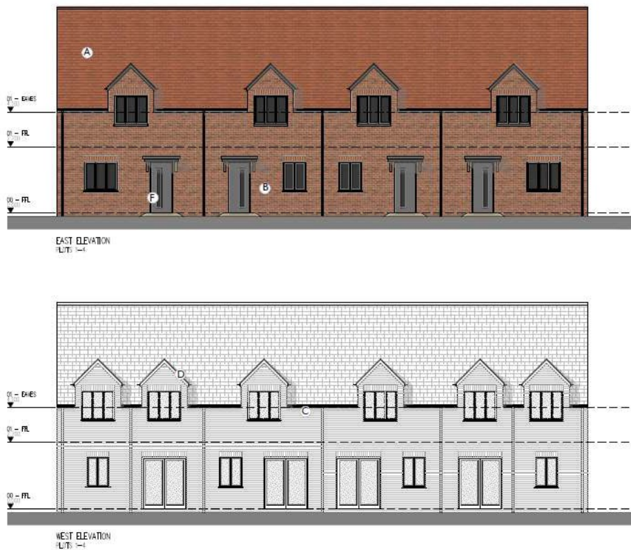
Figure 7: Cottage terrace form: low eaves (and ridge) with through-eaves windows and brick detailing; powder coated composite aluminium / timber windows
